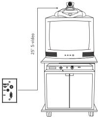
Figure 10. Connection to a video codec
